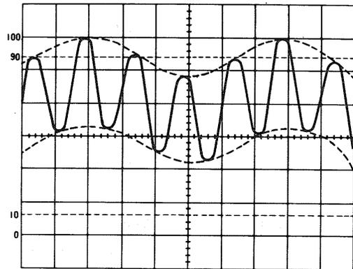
Signal containing undesired component
