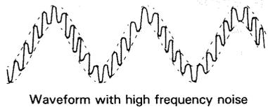
Waveform with high frequency noise
